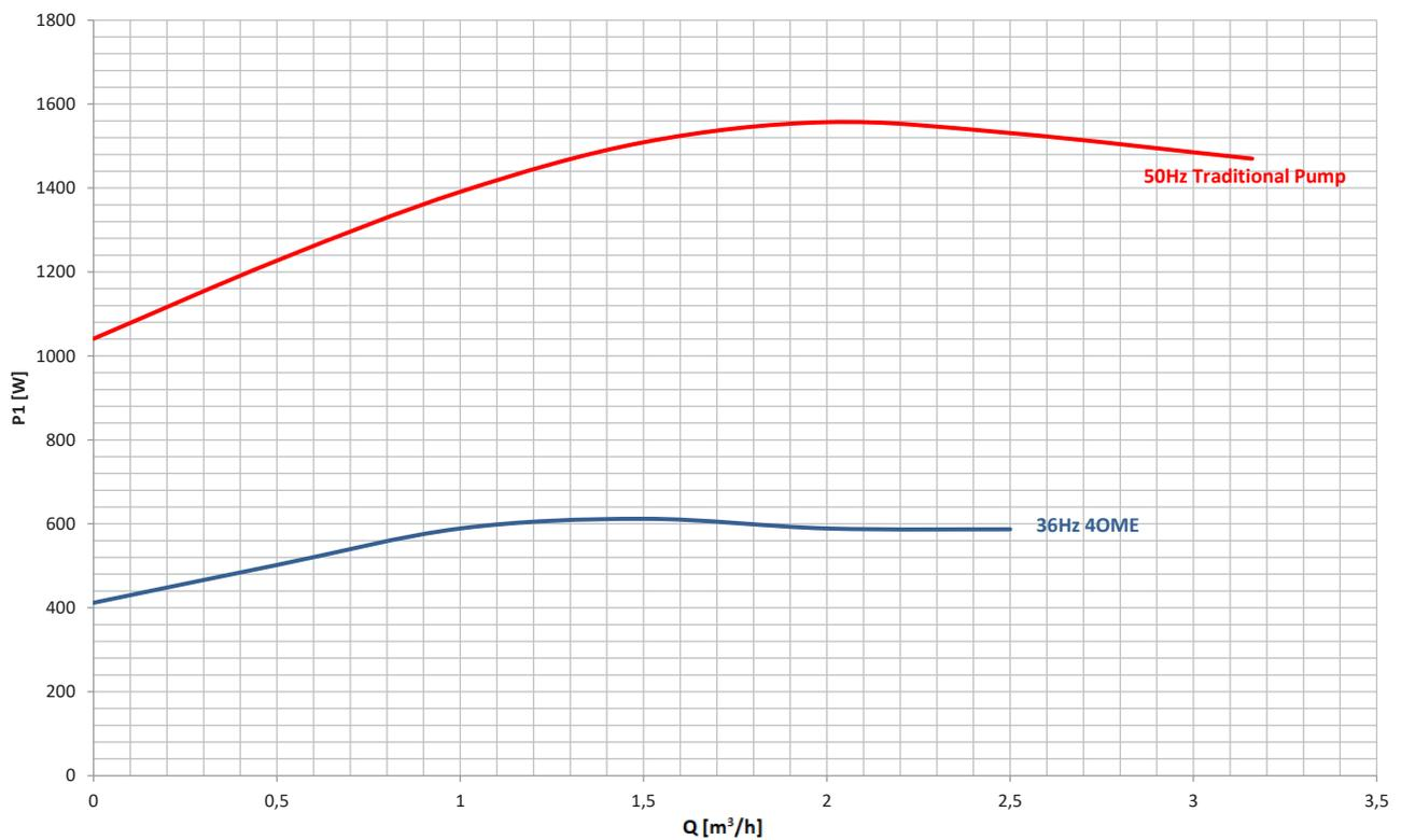
As you can see in the first diagram (Figure 1), the red curve represents a traditional 50Hz pump connected to standard motor without inverter. The blue area is the whole area of use of the same pump connected to the submersible 4OME motor, having 15 - 55Hz as operating range.
