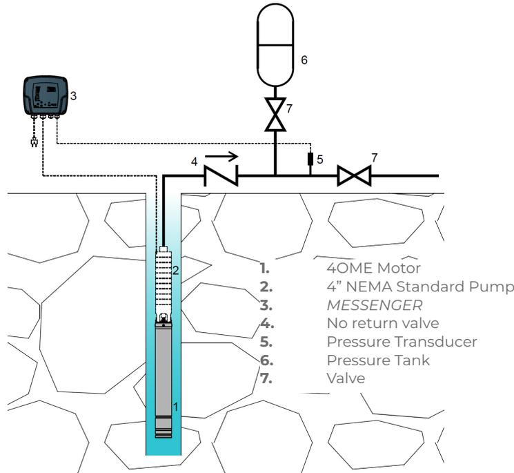
As you can see in the above connection diagram, hydraulic system is considerably simplified too. Indeed you just need to install a small pressure tank and a no return valve in order to keep the plant full of water.
